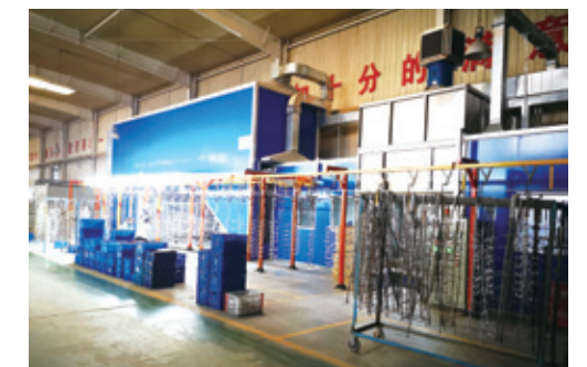
Automatic Painting Line
