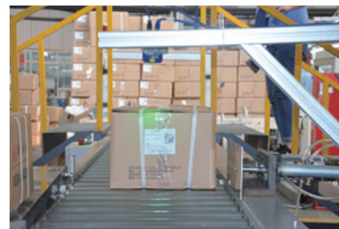
Auto Packing Line with QR Scanning & Identifying storage System
