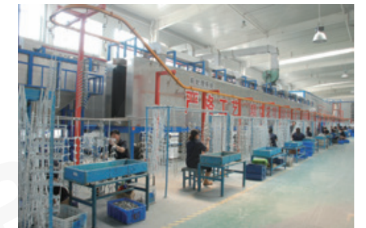
Automatic Powder Coating Line
