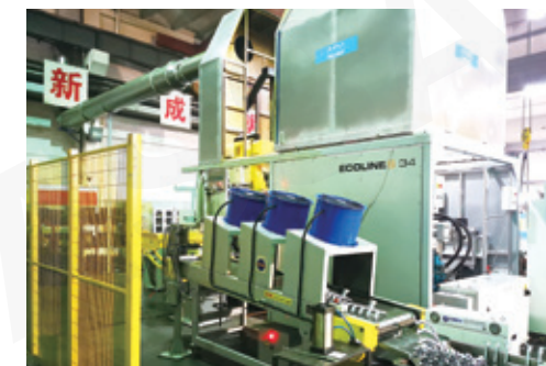
Automatic Alum. Die-casting Machine Swiss brand "BUHLER", 340 tons
